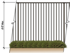
TUBULAR STEEL FENCE COLOR: TBD HEIGHT: 6' MAXIMUM
