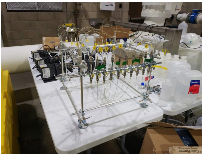
Figure 1. RSSCT column set up
