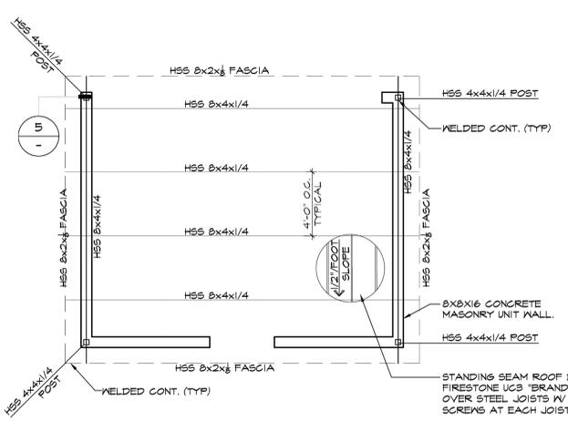
6 TRASH ENCLOSURE ROOF PLAN
