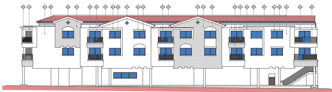
2 EAST ELEVATION-INTERIOR (BUILDING-B) SCALE: 3/16" = 1'-0"
