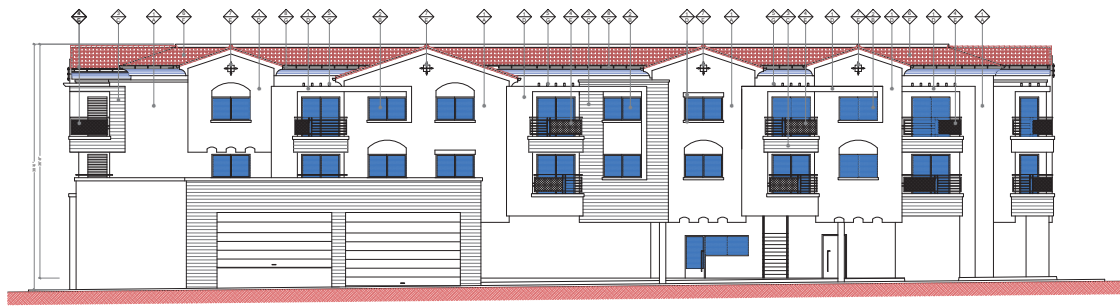
1 WEST ELEVATION-INTERIOR (BUILDING-B) SCALE: 3/16" = 1'-0"
