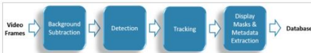
Figure 2. Video Processing Object Extraction diagram.
