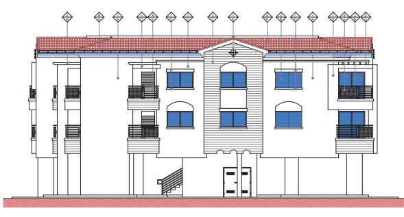
4 SOUTH ELEVATION-INTERIOR (BUILDING-B) SCALE: 3/16" = 1'-0"
