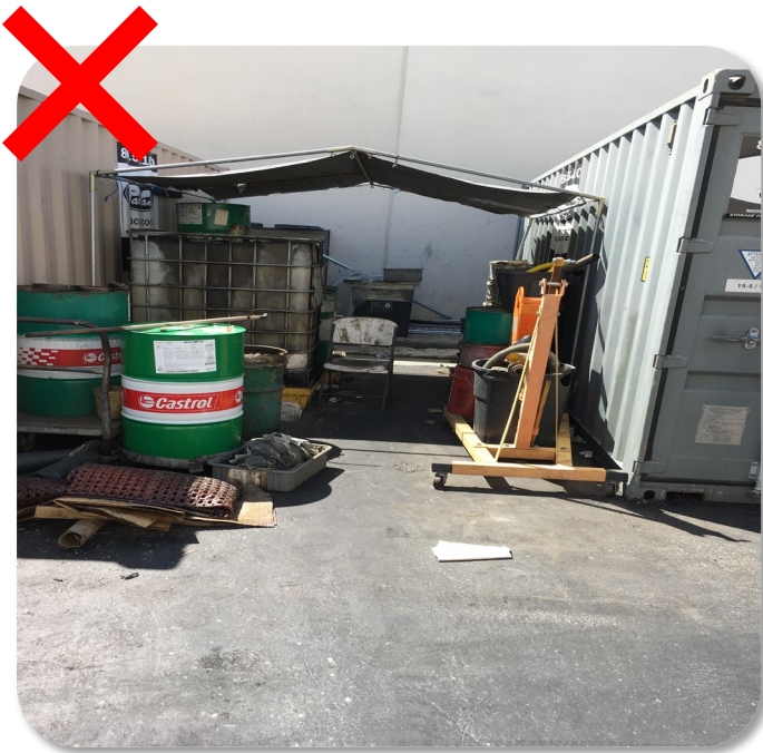
Improper storage containment & cover for materials stored outdoors
