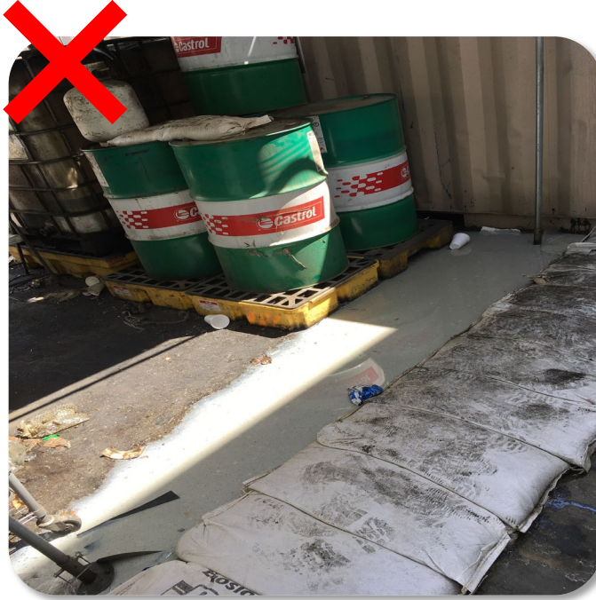
Improper storage containment & cover for materials stored outdoors
