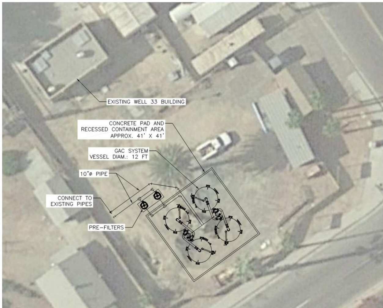
Figure 17. Option 1 – Well 33 Site Layout
